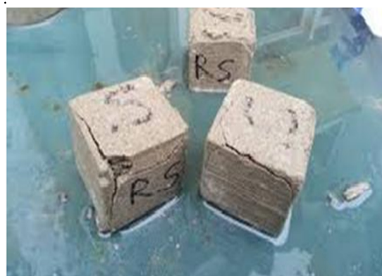
Figure 13: Usual Failure of Concrete At times four vertical faces away leaving two truncated pyramids one inverted over the other. This sometimes accompanied by an explosive sound.
