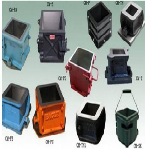
Figure 2: Different types of moulds with different sizes 4.2.TAMPING RODS:
